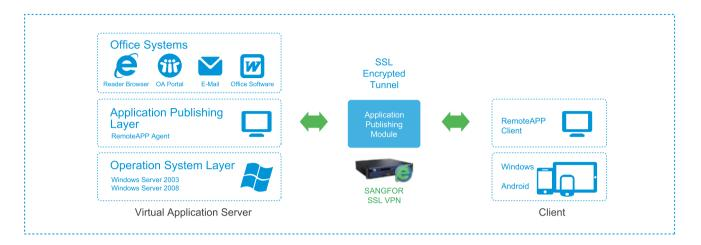
With the remote application enabled, published application interfaces are available on the mobile screens. Thus, users will operate on the virtualized graphical interfaces.
