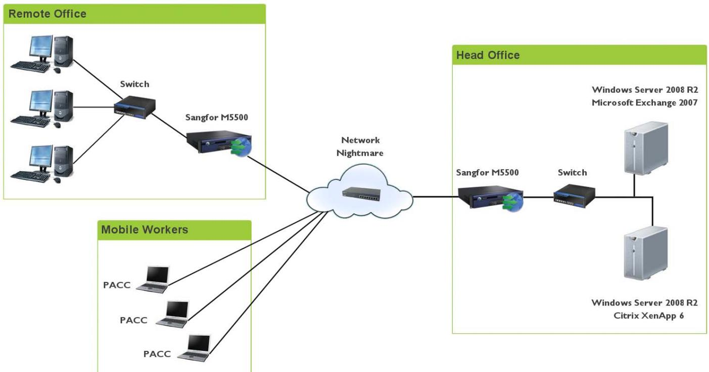
For performance testing we created a network in the lab to simulate an environment comprising a head office and remote site. Two WANACC M5500 appliances were used with one placed in front of the head office network and the other at the remote site.
