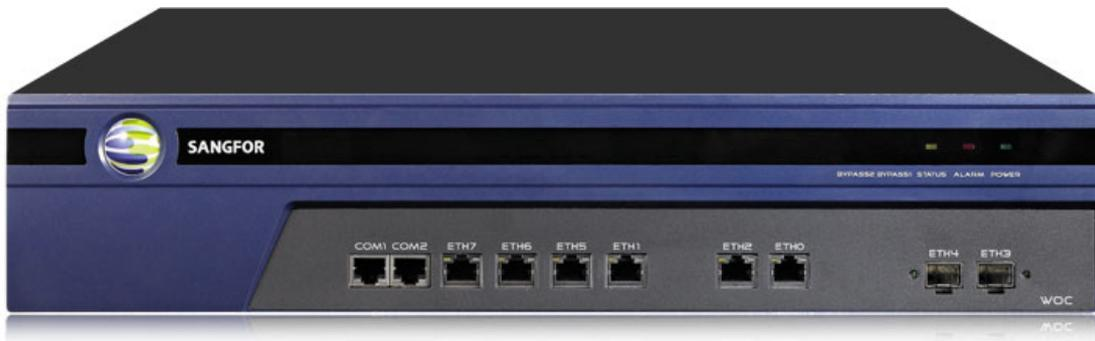
The M5500 appliance on evaluation represents the mid-point of Sangfor's WANACC appliance family and targets deployments in mid-sized businesses and enterprises. It's a well specified 2U rack appliance with a dual-core CPU, 4GB of RAM and four copper Gigabit Ethernet ports which can be used for LAN, WAN and DMZ duties.
